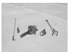
The pike pole can be used to pull material off the roof and also finish knocking any ceiling material after the hole has been cut.
