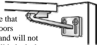
Most types of permanent latches can be installed easily and will not interfere with opening and closing of drawers and doors. The slide lock shown at right can be used on cabinets that do not need to be opened frequently; it is easily installed and removed.
